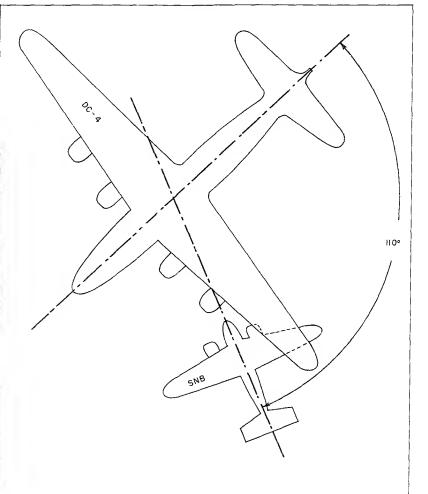
ANGLE OF COLLISION AS DETERMINED BY EXAMINATION OF WRECKAGE CUBANA DC-4 CU-TI88 AND U S NAVY SNB 39939
